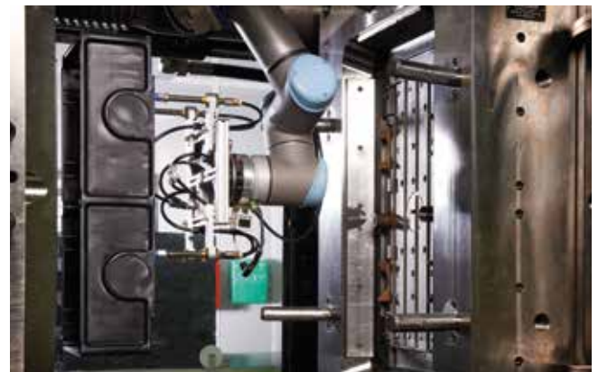
Automatic removal process on VARIABOX injection molding machine
